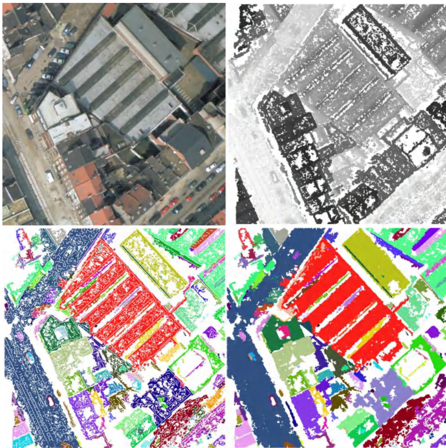
Fig. 3. a) up left : One of the three views of the same area ( 1024 \times 1024 ). Ground resolution is approximately 8\text{cm} \times 8\text{cm} . Courtesy of Eurosense. b) up right : Corresponding disparity map. Darker points are closer to the camera. Unassigned pixels are white. c) down left : Segmentation results after region aggregation. Each segment has a different random color. d) down right : Segmentation results after region merging and hole filling.
