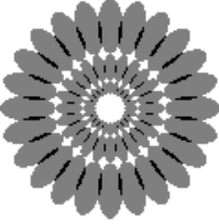
Fig. 1: The applied Gabor filter bank in the frequency domain.
