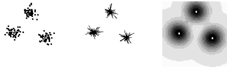
Fig. 3. De-noising of artificial data generated from 3 point sources with Gaussian noise (left), point movements (middle) and contour lines of 'minimal movement' (right).
