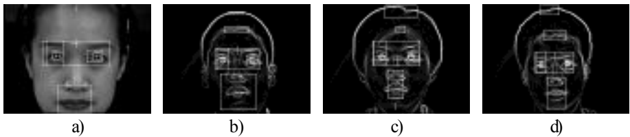
Fig. 13. Face parts extraction windows and detected irises
