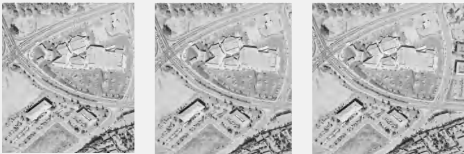
Fig. 3. Original image AERIAL (left) with 8[bpp] and its reconstructions after JPEG (center) with 1.04[bpp] and after KLT (right) with 0.63[bpp].
