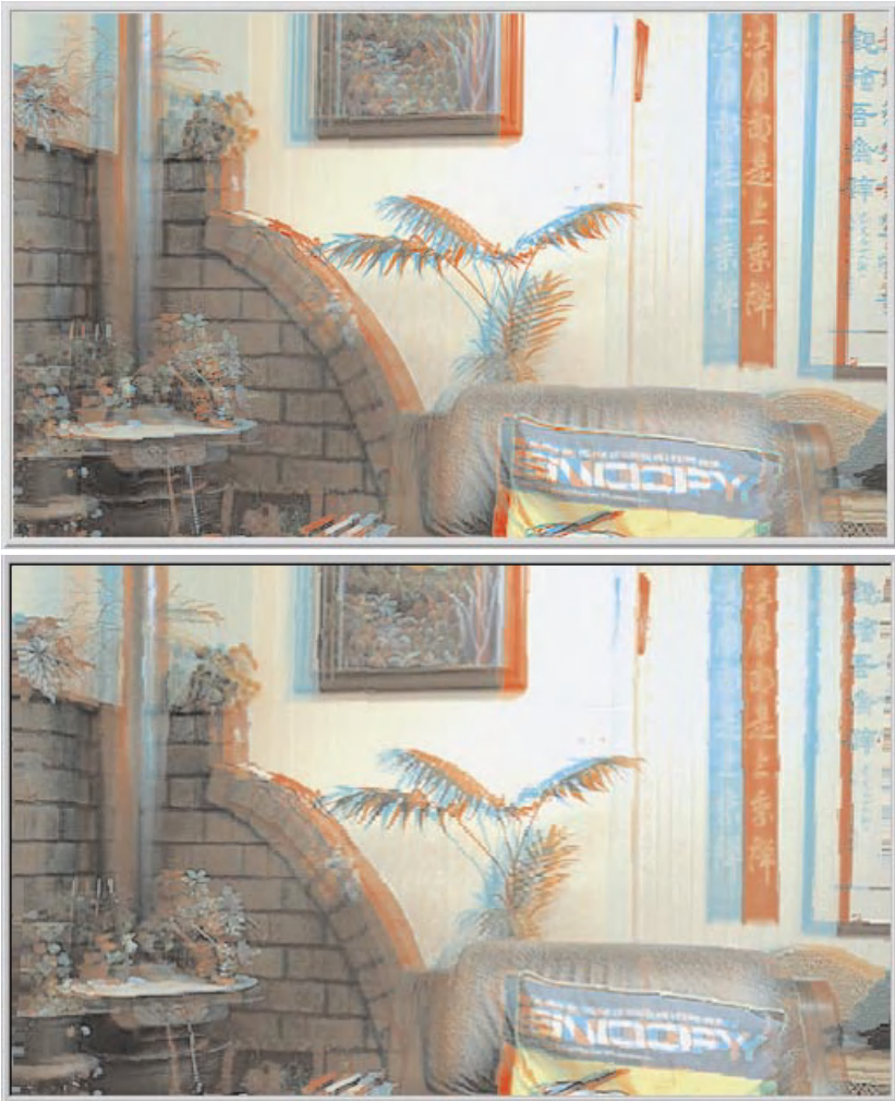
Fig. 4. The top (from our navigator) has crisp vertical borders of objects, while the bottom (from the commercial product) jagged. (See http://www.tcs.auckland.ac.nz/research/projects/demos )
