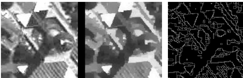
Fig. 4. Berlin Television Tower a) Original b) Smoothed (62 iterations) c) Segment borders
